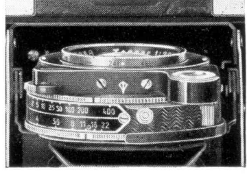
Figures on lens and shutter mounts, visible from above, show distance focused and depth of field.
